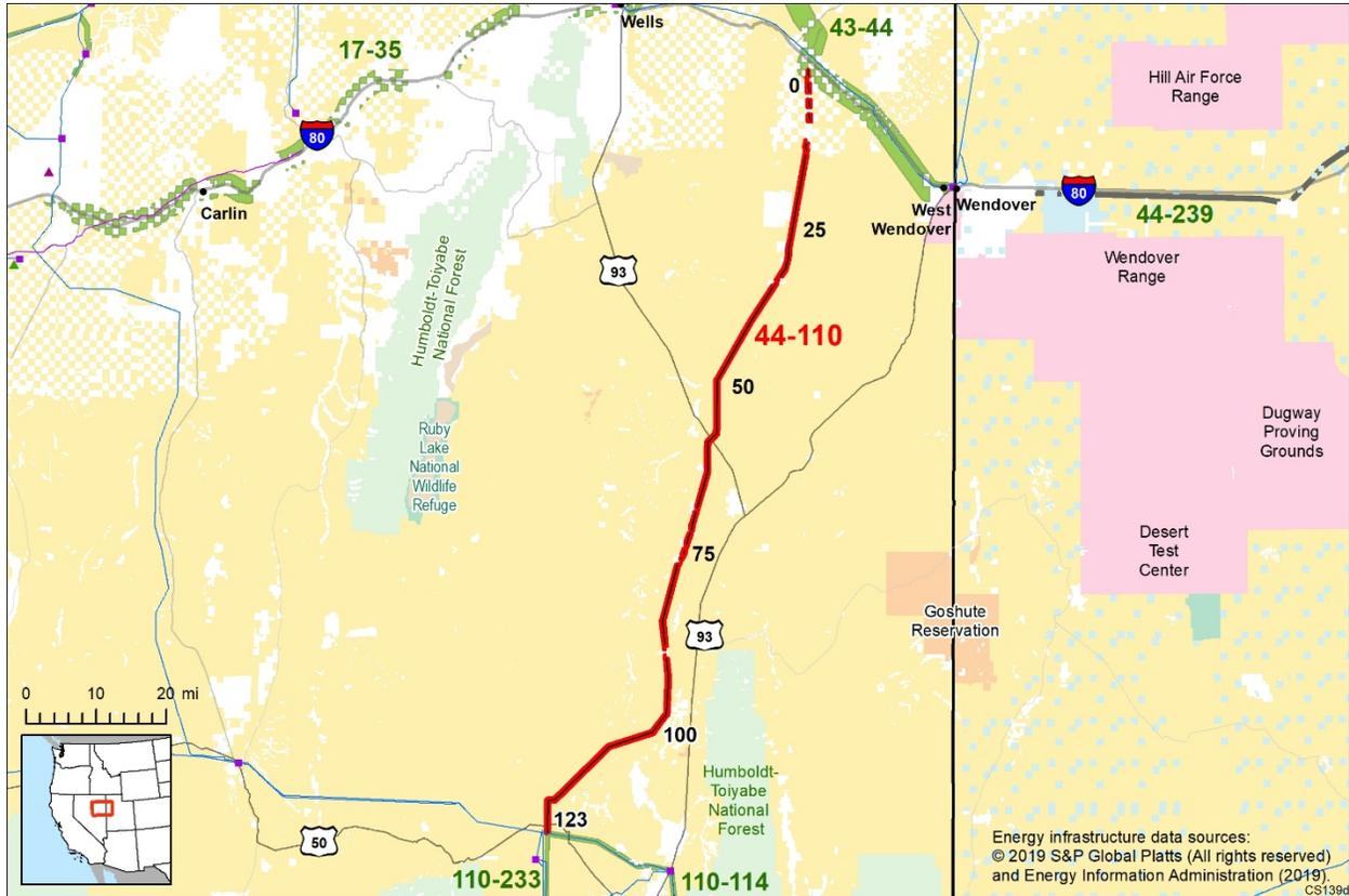
**Figure 3.5-43. Corridor 44-110 and nearby electric transmission lines and pipelines (subject corridor in red).**
