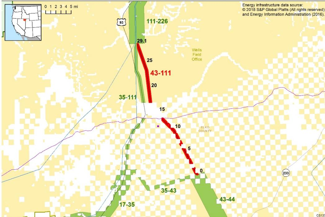
**Figure 3.5-8a. Corridor 43-111 and nearby electric transmission lines and pipelines (subject corridor in red).**
