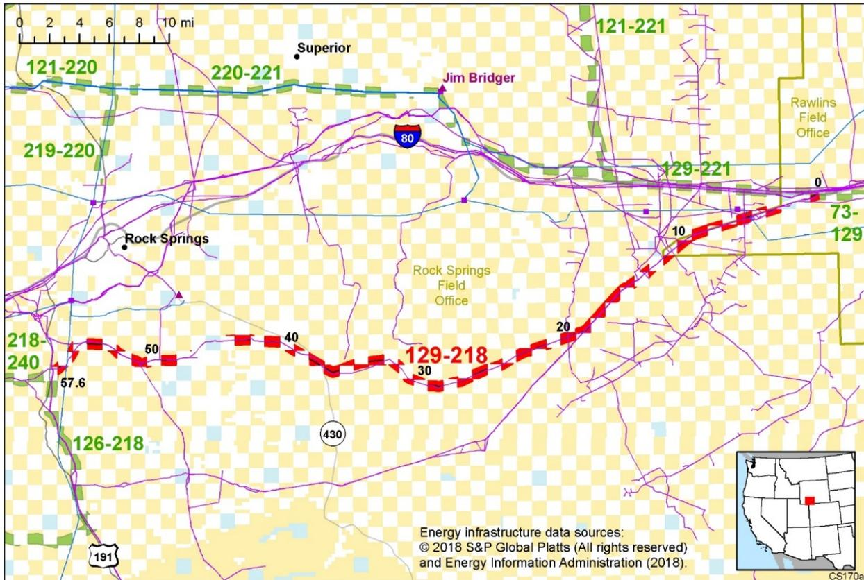
Figure 3.5-48. Corridor 129-218 and nearby electric transmission lines and pipelines (subject corridor in red)
