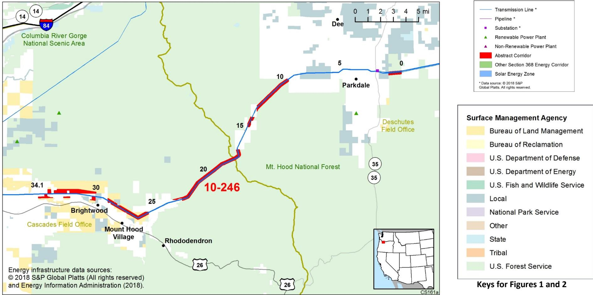
Figure 2. Corridor 10-246 and nearby electric transmission lines and pipelines
