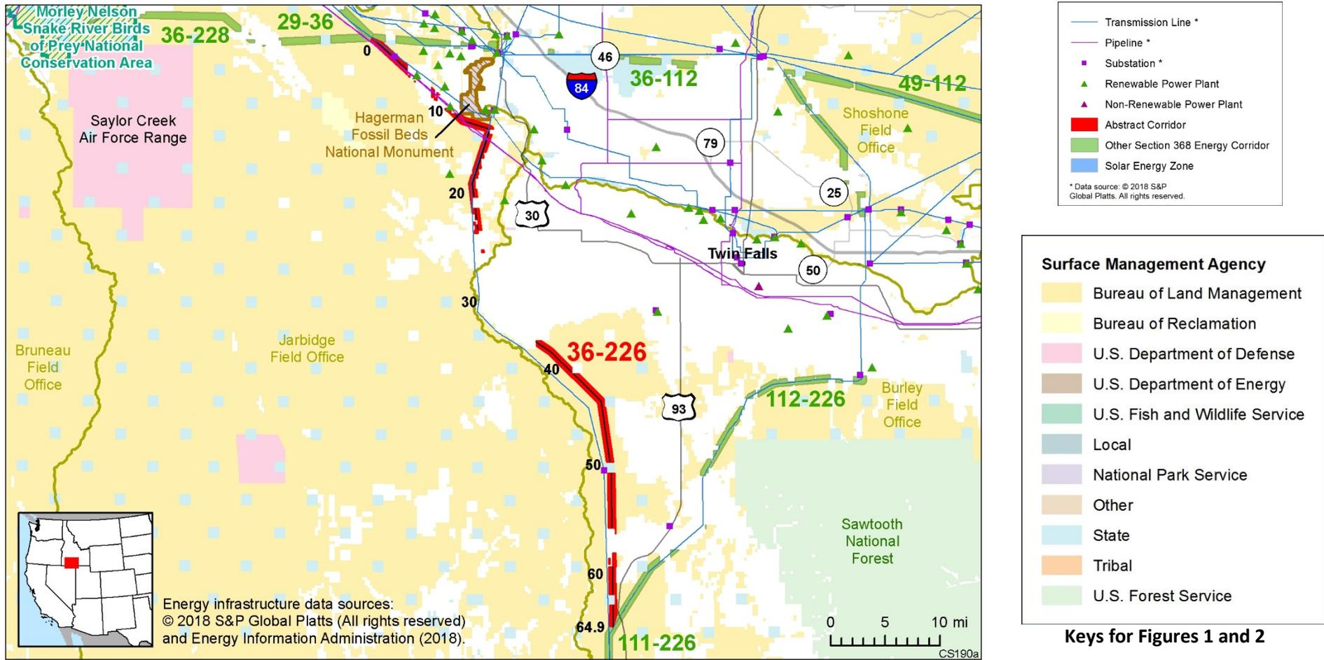
Figure 2. Corridor 36-226 and nearby electric transmission lines and pipelines
